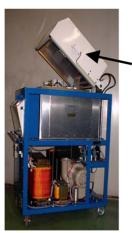
Cabinet inside is completely sealed to prevent dust in mold room when exhaust duct is connected.
