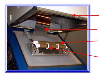
Solid type hood safety bar for consistent obstruction sensing
