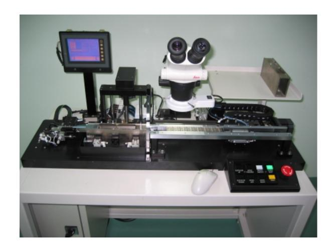
The semi-auto wire bond inspect station that used for lead frame strip inspection. Incorporate with single magazine handling system with a programmable-pitch elevator unit. The lead frame can be index to another position for inspection purposes. The station is equipped with stereo- scope for operator to inspect at any x and y direction of the lead frame.
