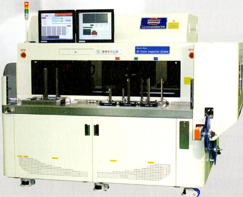
**HANMI 3D VISION INSPECTION** is designed with the latest innovations in vision PMP technology and field proven handler reliability for all types of packages to meet customers' needs : **high productivity, precise inspection, high accuracy, various inspection items, intelligent reject sorting function, easy-to-use user interface and quick change-over.**
